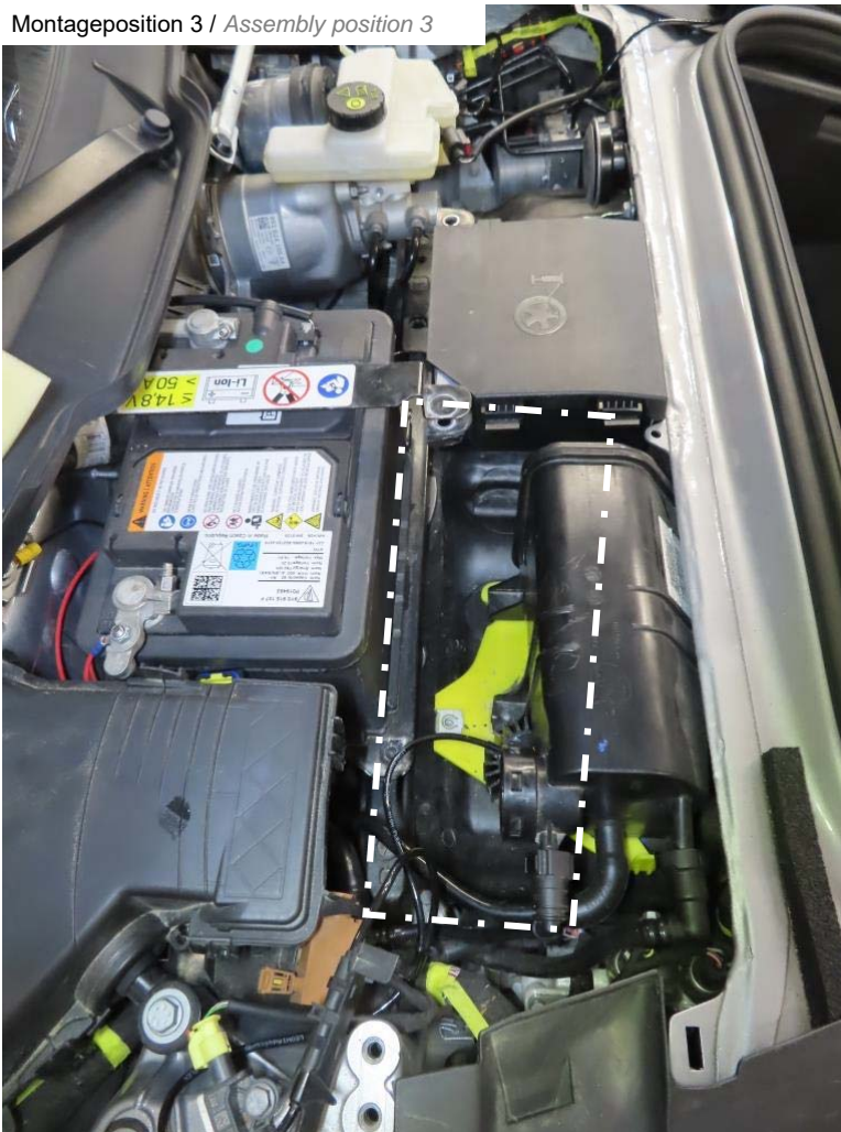
HLS Hydraulikaggregat / HLS hydraulic pump
