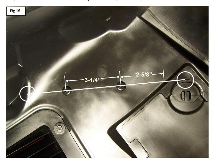
27. Mount the RDC receiver on the front side of the wheelwell liner using the two original rivets with the **connector pointing down**.
