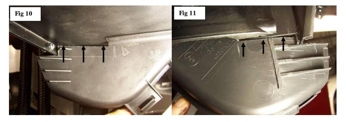
20. Once you have properly fitted the brake duct you can move on to modifying the forward wheel well liner.
