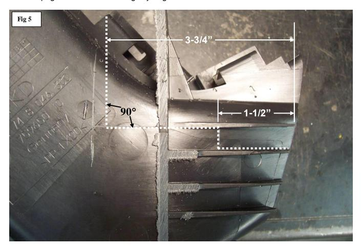
11. Now you can mark the outer side of the right side brake duct. Make the horizontal lines about 1/16" above the "ribs". Note that this duct is already trimmed in the photo.
