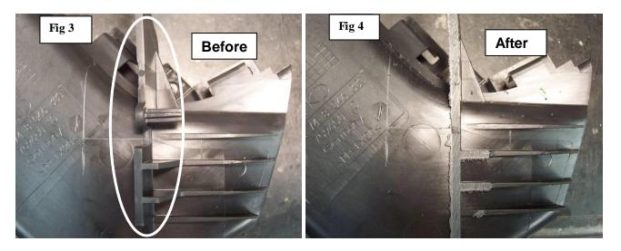
10. Use a small square, a ruler and a sharp scribe to mark the section to be cut on the inner side of the brake duct. Save the silver "captive screw nut" from the piece you cut off. See photo below and next page as well before cutting anything.
