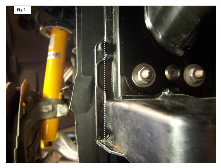
7. Smooth and deburr the cut area where you removed the above edge section. Apply some black touchup paint to any bare metal surface you may have exposed.
