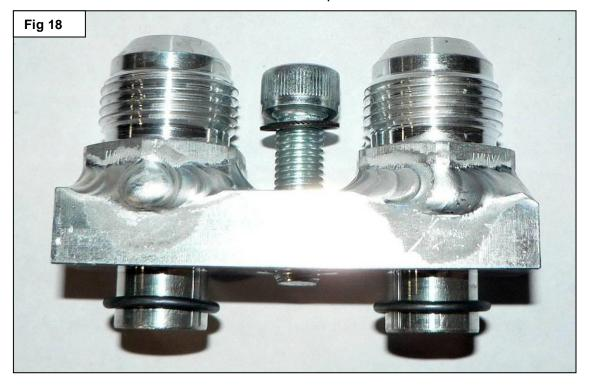
39. Install the Oil Line Mount onto the oil filter thermostat housing. Make sure the O-Rings don't get pinched as you install the block. Hold the Mount up against the thermostat housing firmly as you
