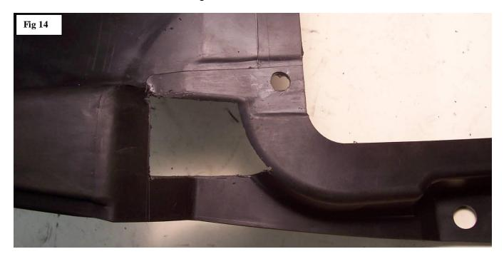
26. You can now relocate the RDC receiver to a higher location on the wheel well liner. Use the photo below to mark a straight line between two points (see circles) then mark and drill two 17/64" holes for mounting the RDC receiver. To prevent the 17/64" drill bit from "wandering" always use a very small bit to drill a pilot hole first. Start the left side of this line roughly at the middle of the curve in the plastic. Note: the receiver is already mounted in place in the photo.
