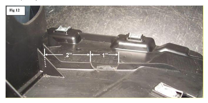
24. Use the photo below to help you measure and mark the small cutout that will allow the wheel well liner to fit around the Oil Cooler.
