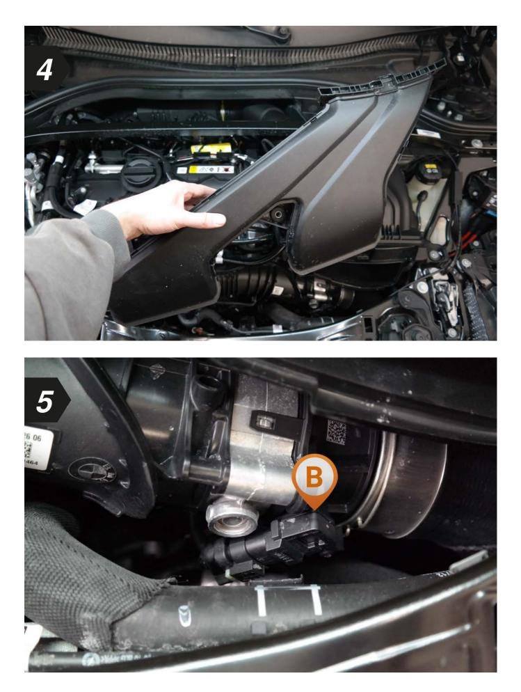
• To begin, locate the turbo boost pressure sensor in your engine bay.
