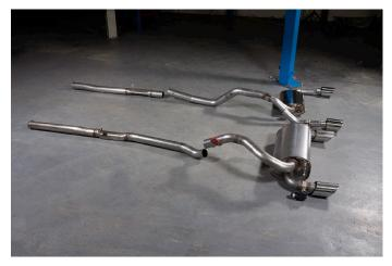
Lay the Scorpion system out next to the original, to help get an understanding of how it will piece together on the car.
