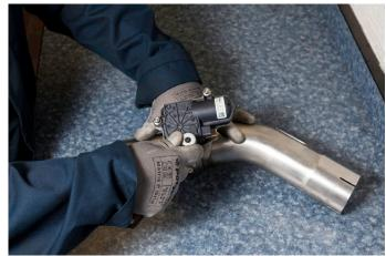
If your vehicle comes fitted with an electronic exhaust valve, you may need to transfer this over from the factory system to the Scorpion. Detailed instructions for this are provided with the product.
