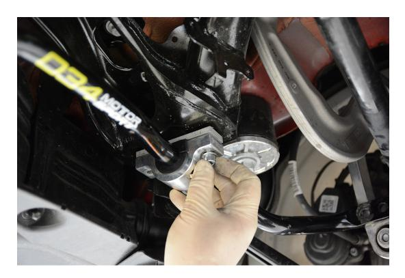
**Step 8** – Attach the sway bar end links to the 034Motorsport Dynamic+ Adjustable Rear Sway Bar using the factory hardware, but do not tighten fully. **Compress suspension to static ride height.** Torque end link hardware to 40 Nm + 180 Degrees.
