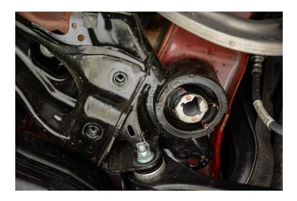
**Step 9** – Apply a thorough coat of grease to the Front 034Motorsport Billet Aluminum Rear Subframe Mount Insert. (PN: 601-0044)
