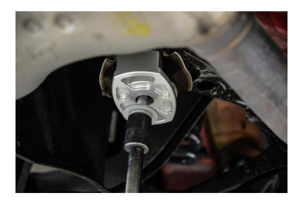
**Step 18 –** Repeat steps 4 through 17 to install the remaining 034Motorsport Billet Aluminum Rear Subframe Inserts for the other side of the rear subframe.
