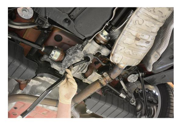
**Step 5** – Using a breaker bar and 21mm socket, loosen and remove the bolt securing the front subframe bushing.
