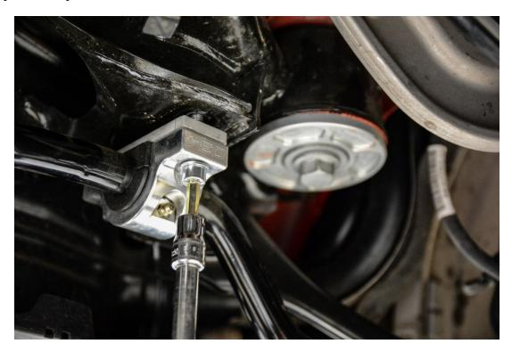
**Step 20 –** Reattach rear sway bar to rear sway bar end links. Torque end link hardware to **40Nm + 180 Degree Turn**. Torque rear sway bar mounting bracket bolts to **28 Nm**.
