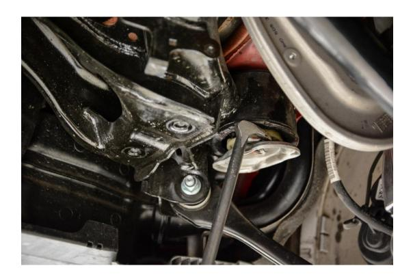
**Step 7** – Finally, remove the factory plastic retainer from the rubber bushing.
