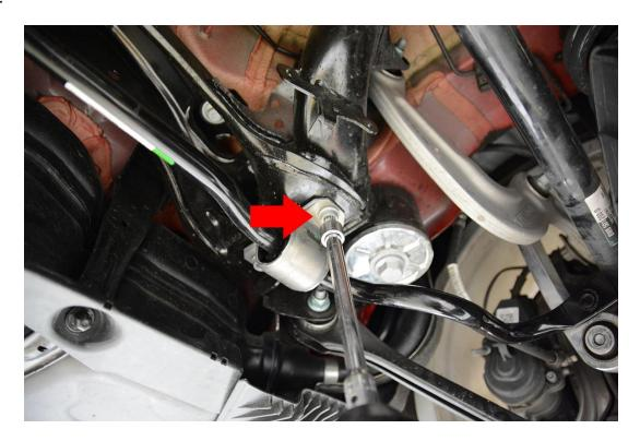
**Step 4** – With the sway bar mounting brackets and end links removed, snake out the rear sway bar from underneath the vehicle.
