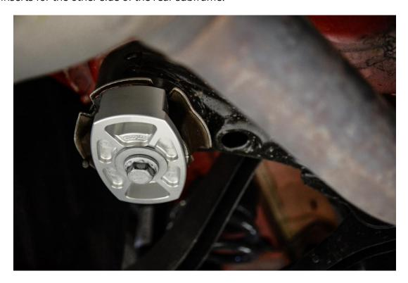
**Step 19 –** Once all four 034Motorsport Billet Aluminum Rear Subframe Inserts are installed and torqued to spec, reinstall the rear sway bar, beginning with the mounting brackets. **Note:** Hardware may differ from factory rear sway bar for aftermarket bars.
