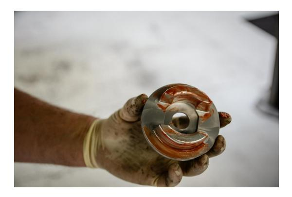
**Step 10** – Insert the Front 034Motorsport Billet Aluminum Rear Subframe Bushing Insert into the factory rubber bushing, and secure using the factory subframe bolt and a 21mm socket.
