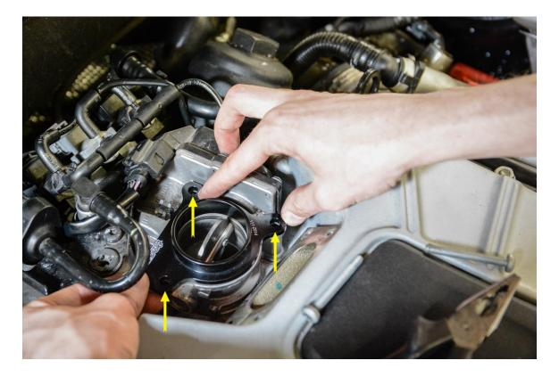
**Step 10** – Place elbow over lip on 034Motorsport Boost Tap and secure 034motorsport Boost Tap to bypass valve with the 3 factory bolts. Use a T30 Torx to snug the 3 factory bolts finger tight.
