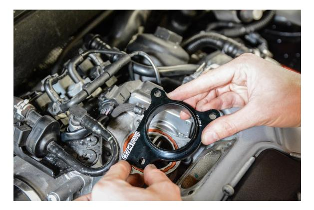
**Step 9** – Place 034Motorsport Boost Tap on top of bypass valve, and align bolt holes.
