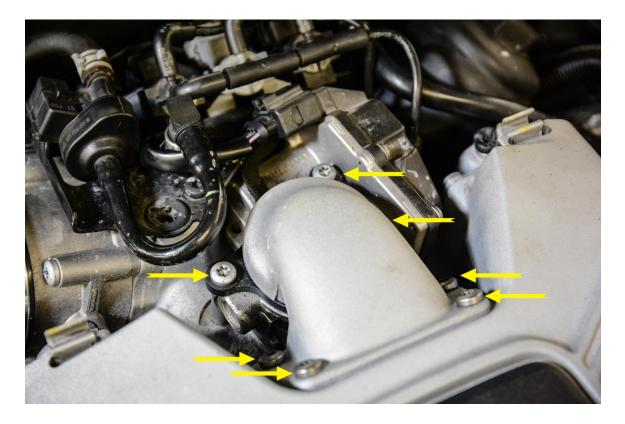
**Step 4** – At this point, 7 bolts should have been removed and the elbow will be free. Lift up to remove elbow from engine.
