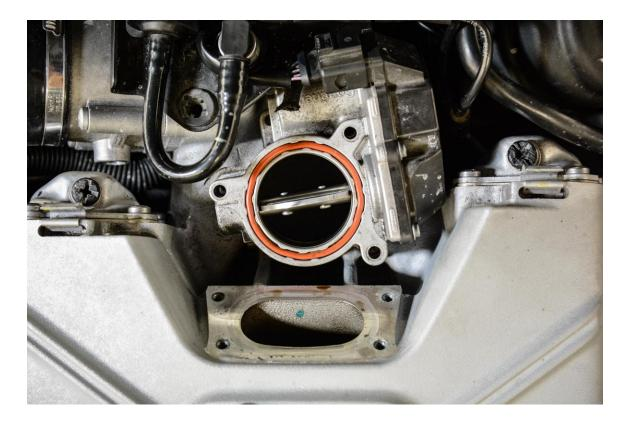
**Step 7** – Using a Small Pry Bar or Flat Head Screwdriver, remove factory plastic plate from the elbow.
