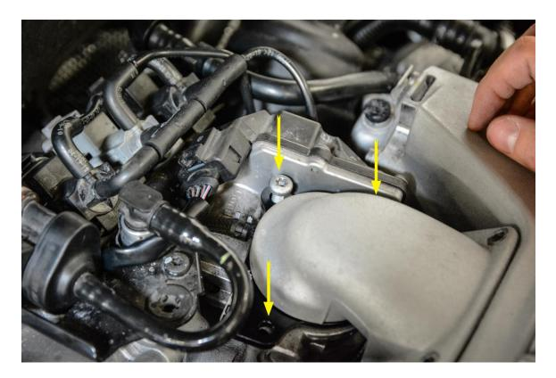
**Step 11** – Secure elbow to supercharger using remaining 4 factory bolts and tighten using a T30 Torx.
