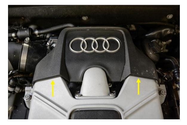
**Step 2** – Using a T30 Torx, remove the 4 Bolts securing the elbow to the supercharger.
