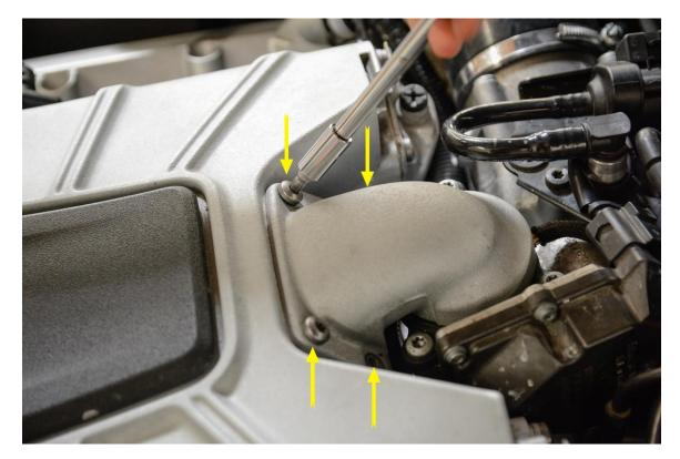
**Step 3** – Using a T30 Torx, remove the 3 Bolts securing the elbow to the bypass valve.
