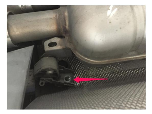
**Step 2** – Remove the triple square bolts securing the factory sway bar mounting brackets to the rear subframe.
