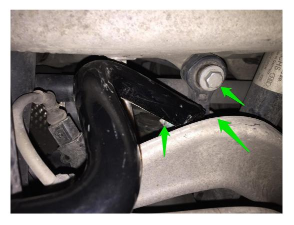
**Step 10** – Tighten the sway bar mount bracket bolts to 28 Nm.
