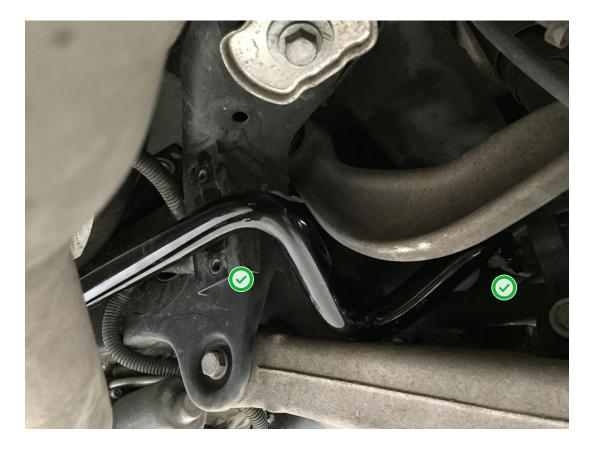
**Step 6** – After applying the supplied grease, install the polyurethane sway bar bushings onto the bar as shown.
