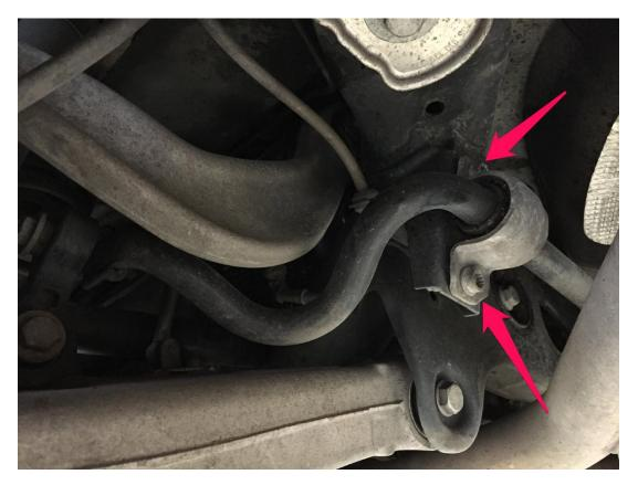
**Step 3** – Remove the rear sway bar end link bolts and nuts, and remove the rear sway bar end links. With the end links removed, snake out the rear sway bar from underneath the vehicle.
