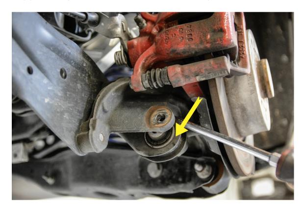
**Step 8** – Remove the factory toe link completely from the car.
