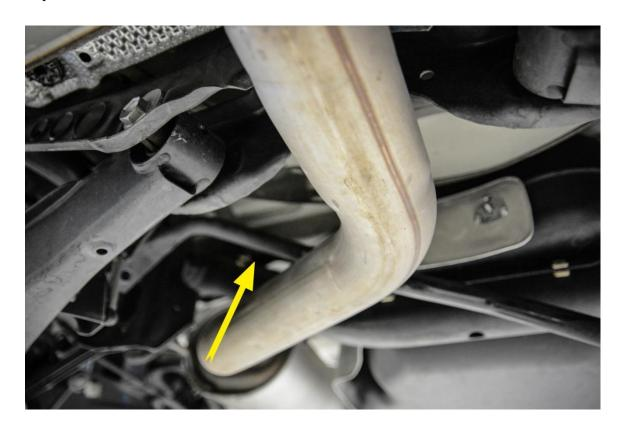
**Step 6** – Using the same technique, rotate and position the new 034Motorsport Mk5/Mk6 FWD rear sway bar underneath the car. **Careful** not to hit the exhaust when getting the sway bar in position.
