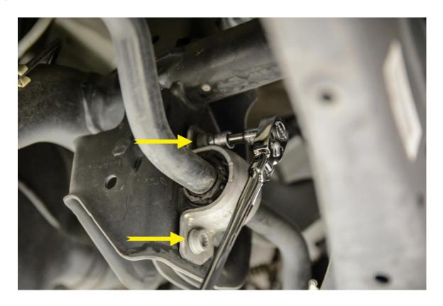
**Step 5** –Remove the factory sway bar from the car, careful to rotate it around the exhaust. install the 034Motorsport Solid Rear Sway Bar.
