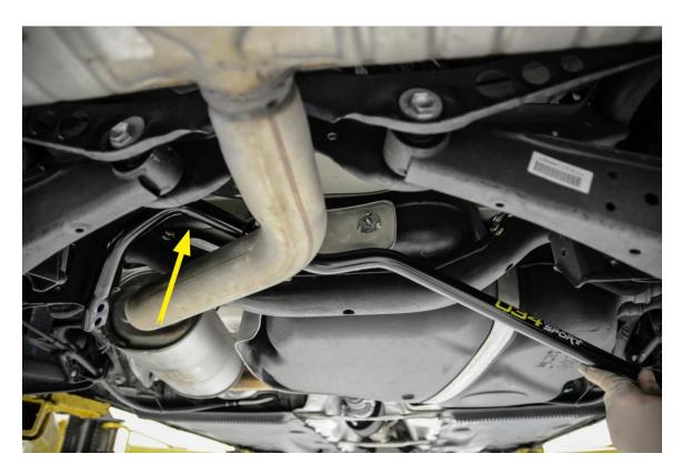
**Step 7** – Grease and install the supplied Polyurethane Sway Bar Bushings onto your 034Motorsport Solid Rear Sway Bar Upgrade as shown below.
