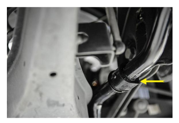
**Step 8** – Prepare to install the Billet Aluminum Sway Bar Mounts, and apply a small amount of blue loctite to each of the supplied M8 bolts.
