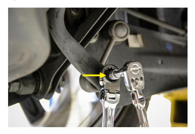
**Step 3** – Once the nut is free from each of the sway bar end links, rotate the sway bar so that it is free from each end link.
