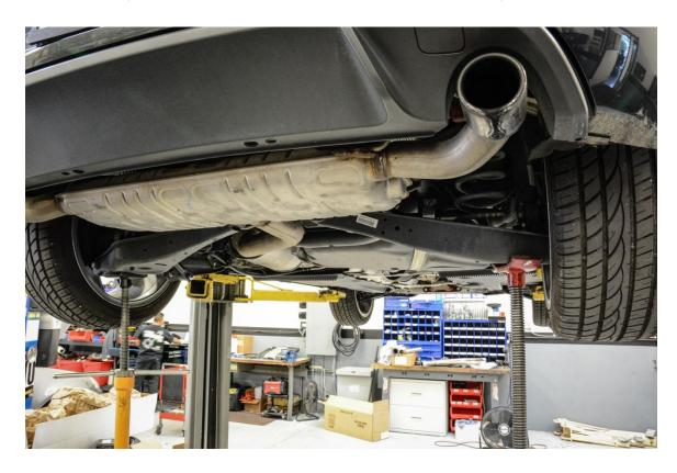
**Step 2** – Using a 16mm wrench and 6mm triple square, remove the nut securing each of the rear sway bar end links to the rear sway bar.
