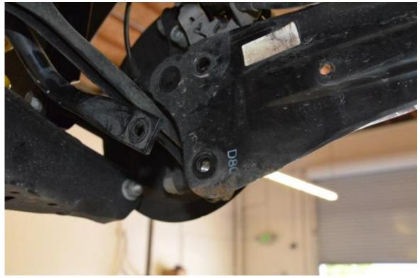
**Step 6** – Remove the four 16mm bolts holding the trailing arm housing to the chassis.
