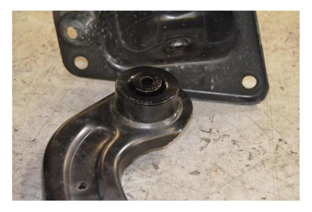
**Step 12** – Install new 034Motorsport arm into housing, and install 18mm bolt. Torque to 90Nm + 45 degrees. **DO NOT OVERTIGHTEN!** Overtightening can cause the spherical to bind!
