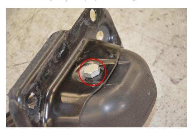
**Step 10 –** Trailing arm and housing should be separated now. Discard old trailing arm, and identify correct replacement from 034Motorsport Spherical Rear Trailing Arm Pair.
