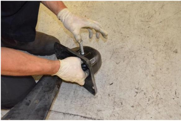
**Step 13** – Begin to reinstall arm and housing assembly into the vehicle. Use one bolt at each end to line up. You may have to push up on the upright and/or compress the suspension slightly to align all holes.
