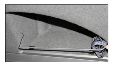
Lift down the grille out of its holding and push the grid to the side. Rotate the retaining clip by 90 degrees and than pull out the grille.
