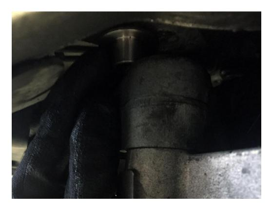
**Step 10** – Install the bottom locking collars into the subframe, and thread in the supplied M12x110mm bolts a few turns to hold up the subframe while you install the remaining two collars.
