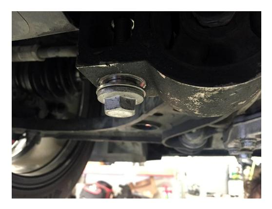
**Step 8** – Using an 18mm socket, remove both rear subframe bolts, which are probably bent. These will be replaced with the supplied constant-diameter M12x110mm subframe bolts once the locking collars are installed.
