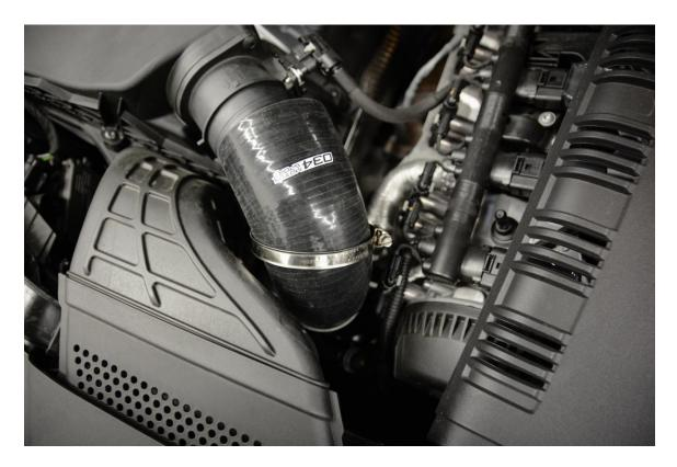
**Step 8** – Using an 8mm socket, tighten the upper and lower hose clamps to secure the 034Motorsport High Flow Silicone Turbo Inlet Hose.
