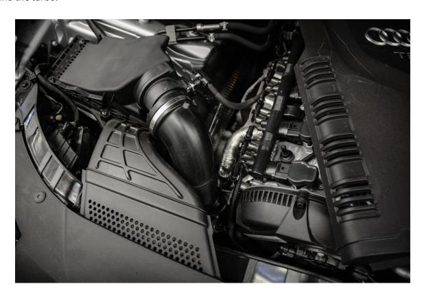
**Step 4** – With both clamps loosened, remove the factory turbo inlet hose from the engine bay and notice how restrictive and ugly it looks.
