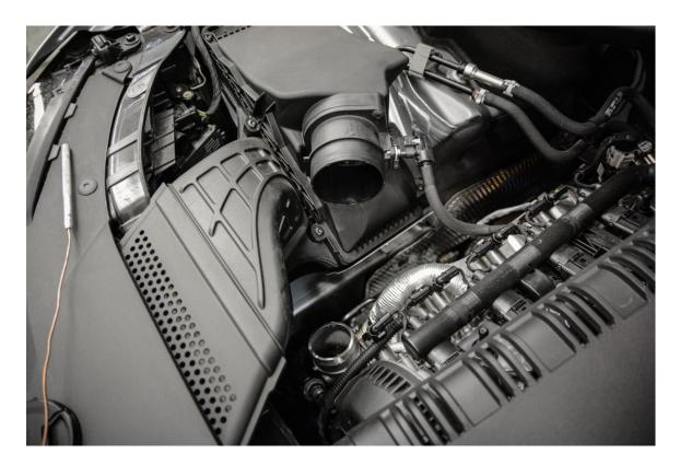
**Step 7** – Position the 034Motorsport High Flow Silicone Turbo Inlet Hose such that the narrower portion is over the turbo inlet, and the larger opening mates to the MAF housing.
