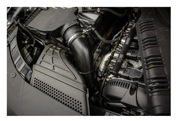
**Step 3** – Using a 7mm socket, loosen the upper and lower hose clamps securing the factory turbo inlet hose to the air box and the turbo.
