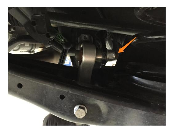
**Step 8** – With the sway bar properly aligned, install the supplied Billet Aluminum Sway Bar Mounts with the zerk fitting pointing down. Secure using the supplied M8 Bolts & Washers. Torque to 28 Nm.
