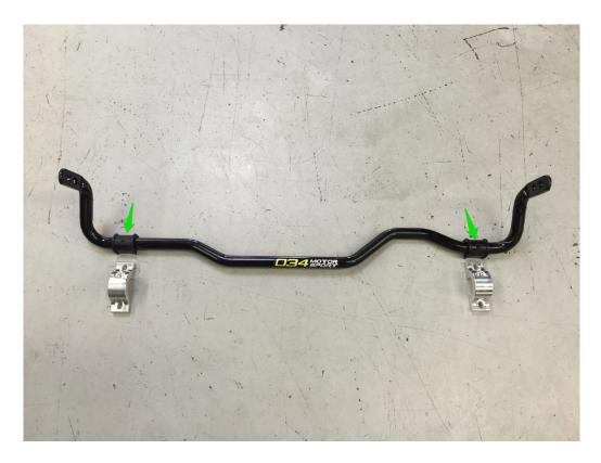
**Step 7** – With the sway bar in place, reinstall the nuts to the factory rear end links, or install your new MQB Spherical Rear Sway Bar End Links if you purchased those as well. Torque the stock hardware to 35 Nm.
