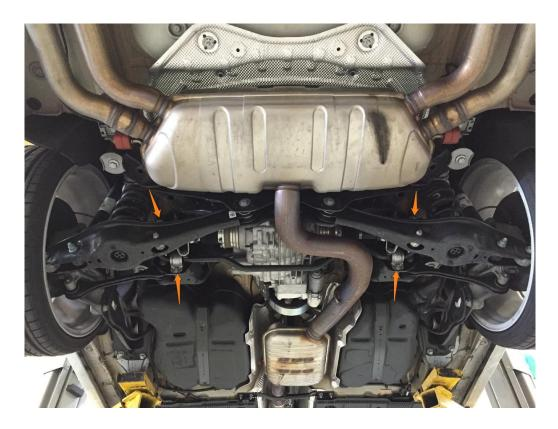
**Step 2** – Using the 10mm Triple Square, remove the two M8 Bolts securing each of the factory rear sway bar mounting brackets to the subframe.
