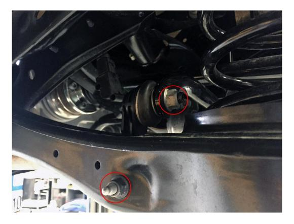
**Step 2** – Using two 13mm wrenches, remove the bolt and nut securing the bottom of the end link to the lower control arm. Using a 16mm wrench and 6mm triple square, remove the nut securing the upper end link to the rear sway bar.
