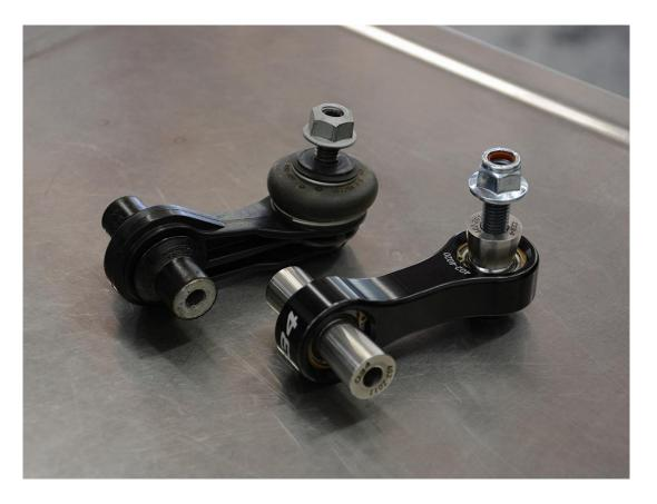
**Step 4** – Install the 034Motorsport End Link into the lower control arm with the two long spacers at the bottom. Secure using the factory bolt and supplied M8 lock nut. Torque to 35 Nm.
