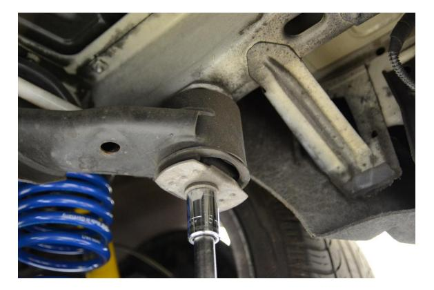
**Step 3** – Once the subframe bolt is removed, use a small pry bar to separate the factory washer from the rubber bushing.
