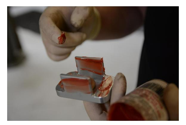
**Step 6** – Align the 034Motorsport Rear Subframe Insert (601-0040) with the voids in the factory subframe bushing. Install subframe bolt using an 18mm Socket. **Note:** We recommend replacing the original subframe bolts with new pieces, as they are stretch bolts that are intended for a one-time use.
