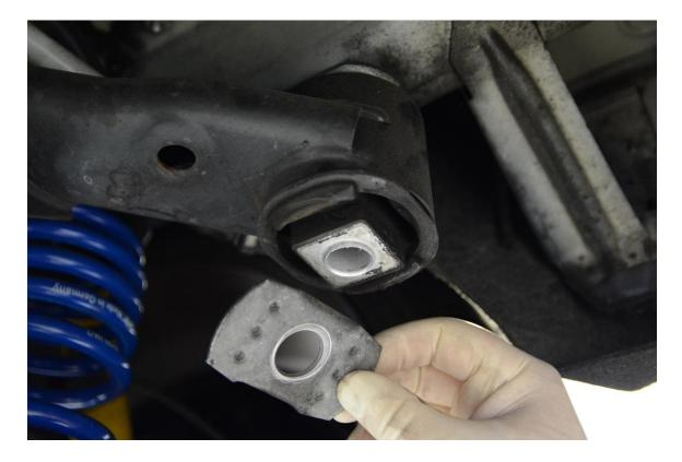
**Step 5** –Apply silicone grease to the insert as pictured below.
