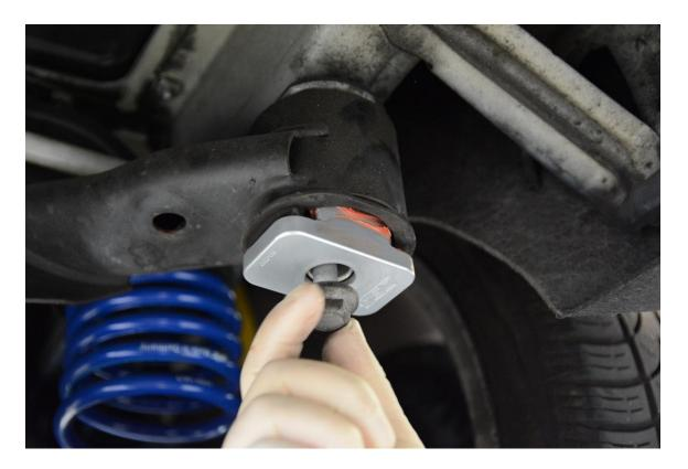
**Step 7** – Torque new subframe bolt to 90 Nm + 90° Turn. **If you opt to reuse the stock bolts, torque them to 90 Nm with Blue Loctite.**
