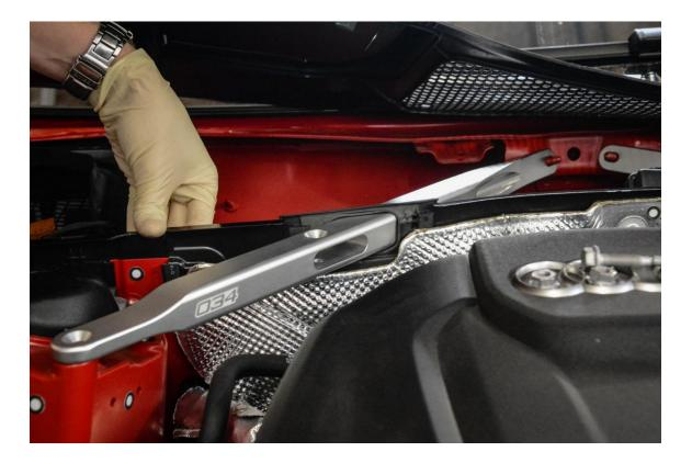
**Step 16 –** Loosely install both factory rear mounting nuts.
