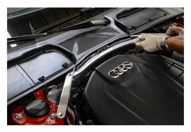
**Step 18** – Using a 5mm Allen Key and 2 of the supplied M8 flathead screws, secure the cross brace to the left and right strut brace. Torque to **35 Nm.**
