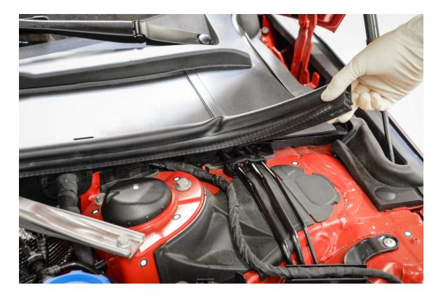
**Step 3** – Once removed, place the rubber seal to the side, as this will need to be installed later.
