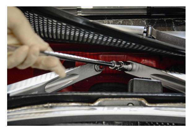
**Step 20 –** Install the remaining 2 supplied M8 flathead bolts to the left and right strut brace, securing the brace to the strut tower. Torque to **25 Nm.**
