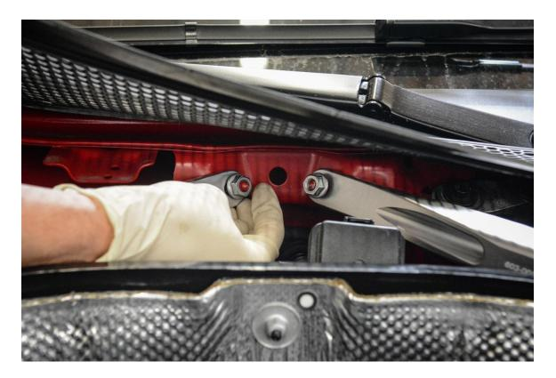
**Step 17** –Noting the orientation, insert the ends of the billet aluminum cross brace into the slots of both left and right strut brace.
