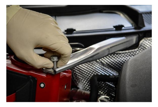
**Step 8** – With the same 13mm socket, remove the front mounting bolt for the driver side strut brace.
