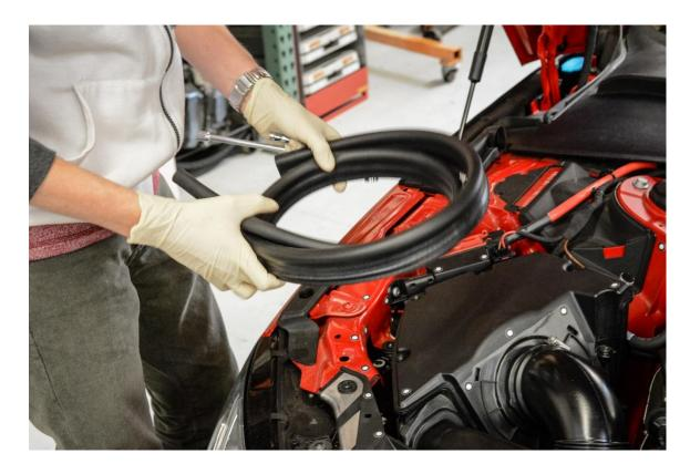
**Step 4** – Lift up on the plastic cowl cover to locate the 2 rear mounting nuts for the factory strut braces.
