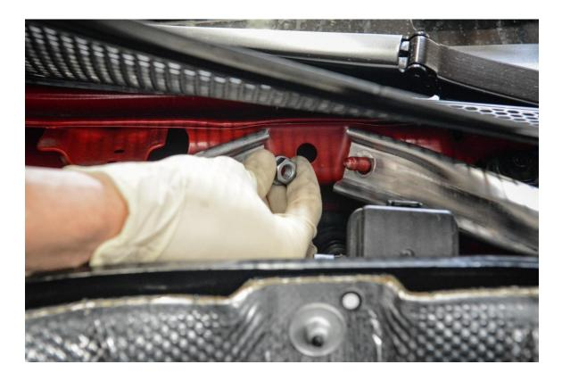
**Step 7** – Using a 13mm socket, remove the front mounting bolt for the passenger side strut brace.
