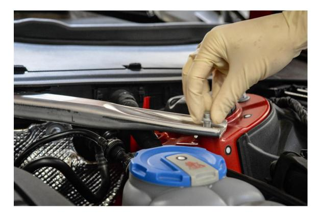
**Step 9** – Once all mounting hardware has been removed, lift up vertically on the factory brace and plastic trim to free it from the chassis.
