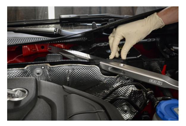
**Step 14 –** Once properly installed, the plastic trim should sit flush with the firewall.
