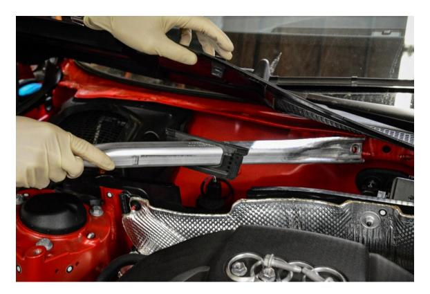
**Step 11** – Compare the factory stamped metal braces to your robust 034Motorsport Billet Aluminum Strut Brace and identify the left and right specific braces.
