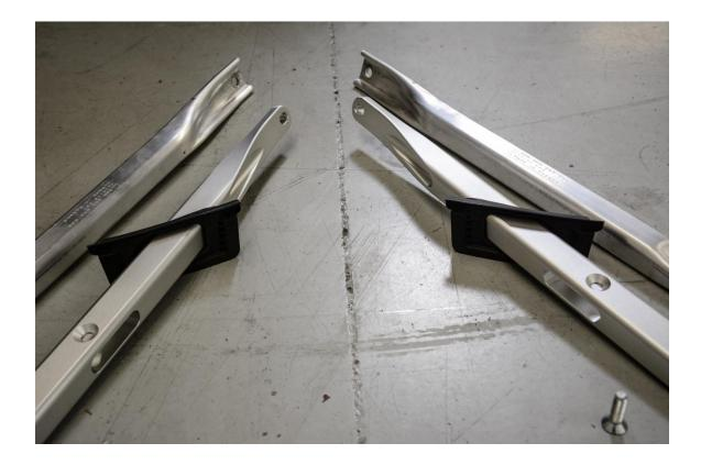
**Step 13 –** Install the driver side billet aluminum brace (603-0013), careful to line up the plastic trim with the firewall.
