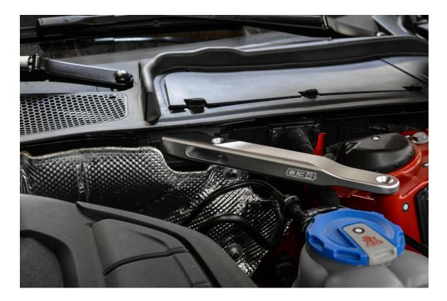
**Step 15** – Follow the same procedure for the passenger side (603-0014), making sure to line up the rear mounting stud with the hole and securing the trim to the firewall.
