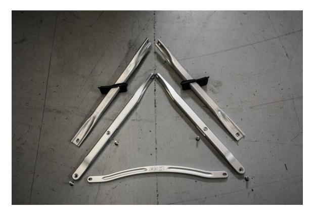
**Step 12 –** Transfer the factory plastic trim from the OE braces to your new 034Motorsport billet aluminum braces.
