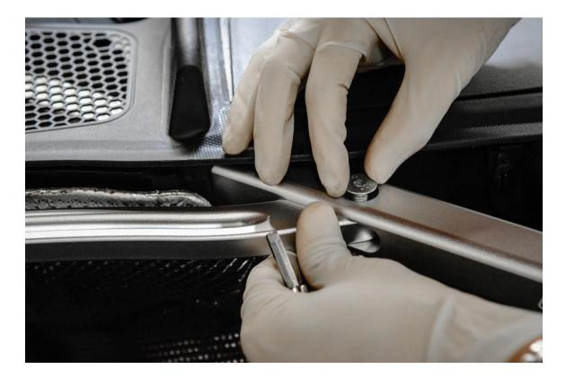
Step 19 – Tighten the factory nuts to rear mounting points. Torque to 20 Nm.
