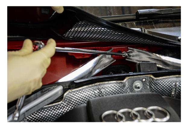
**Step 6** – Keep these nuts in a safe place, as they will be used to install the 034Motorsport Billet Aluminum Front Strut Brace.
