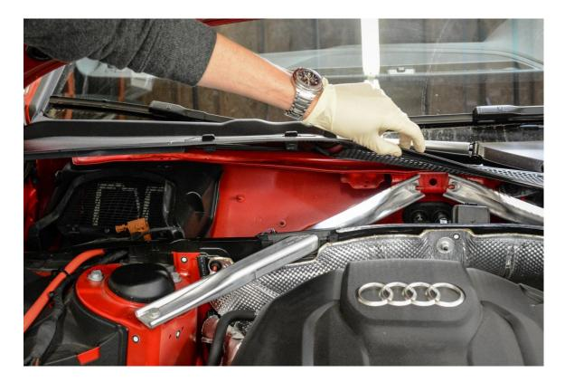
**Step 5** –Using a 13mm socket, remove the left and right rear mounting nuts for the factory strut brace.
