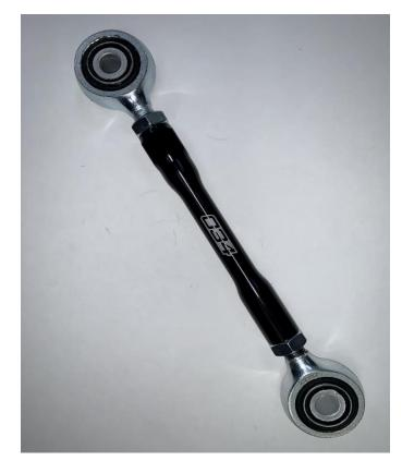
You are now ready to start the installation process. Use the length of the stock component as a starting point for the length of the 034 adjustable end links; expand or compress as best fits your needs
