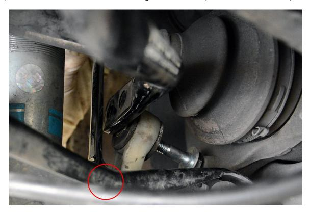
**Step 3** – This step will require some patience, and small hands help as well. If you have a patient friend with small hands, give him a call and invite him over to help. With a spacer installed on each side, secure the bottom of the Spherical Sway Bar End Link to the lower control arm with the supplied M10x50 Bolt and M10 Washer. Torque to 55 Nm.
