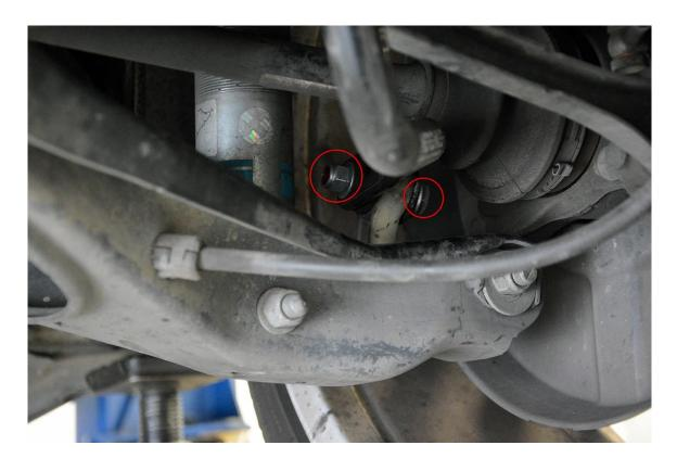
**Step 2** – Using a 15mm wrench, remove the bolt securing the bottom of the end link to the lower control arm. This is a tight space, but the bolt can be removed without touching the rest of the suspension. Remove the factory end link.
