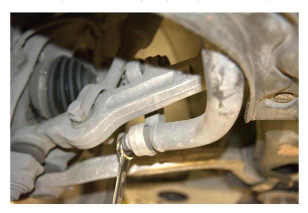
**Step 3** – Using the 16mm wrench, remove the upper end link bolts from the front sway bar end links. If needed, you can use the 13mm wrench to counter hold the nut on the other side.
