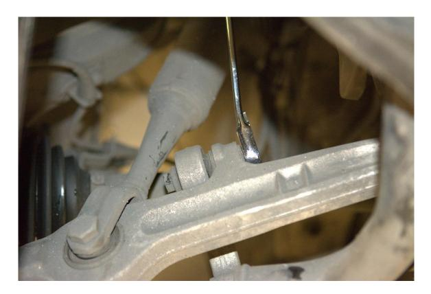
**Step 4** – Remove the factory front sway bar end links. Pat yourself on the back; you're halfway done! With the stock end links removed, the 034Motorsport Billet Aluminum Spherical Front Sway Bar End Links can be installed using the supplied hardware. You'll need a 16mm wrench for the supplied bolts and 15mm wrench for the supplied locknuts.
