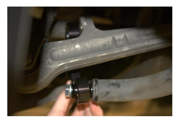
**Step 7** – Install the supplied M10x65 bolts through the lower control arms and the tops of the end links, with the supplied washers between the bolts and control arms. Secure the bolts using the supplied M10 locknuts.
