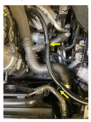
**Step 13** – Install the catch can assembly using the screws removed in Step 9. Install second hose clamp onto the silicone hose and attached to banjo. Tighten hose clamp:
