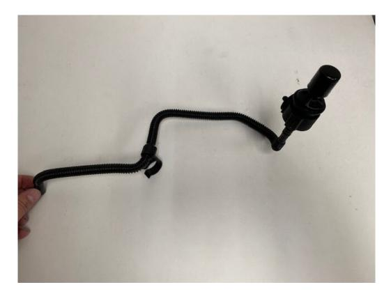
**Step 7** – Install the banjo fitting onto the catch can, with an aluminum crush wash on either side of the banjo fitting.
