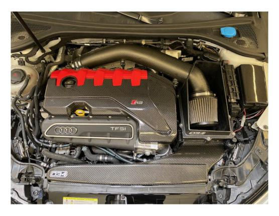
**Step 2** – Unclip the factor "catch can" from the airbox:
