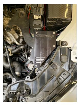
**Step14** – Reinstall intake (removed in Step 3). Step back, admire your work, and rejoice that you will no longer have DSG fluid all over your engine bay!
