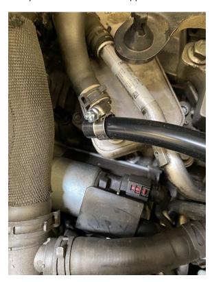
**Step 11** – Put this end of the hose onto the transmission breather connection, and using a 7mm socket, or Philips head screwdriver, tighten the hose clamp:
