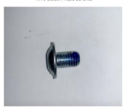
**Step J**Torque to 25 Nm with a 6mm Allen
