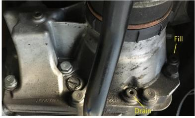
**Step 3** Using a 5mm Allen bit, remove both plugs.
