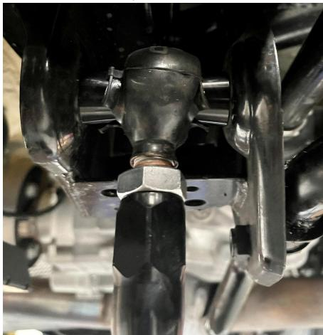
**Note**: Use the short spacers are on the hub assembly and the taller spacers on the rear subframe. To make adjusting easier, the hex end of the tube should connect to the subframe.
