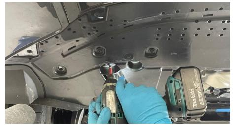
**Step 5** Using a T30 Torx, remove the hardware for the side underbody panels in the wheel well.
