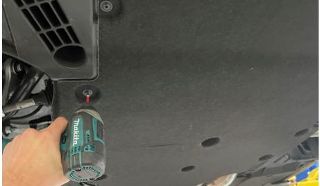
**Step 4** Using a T20 Torx and 13mm socket, remove the hardware for the side underbody panels.
