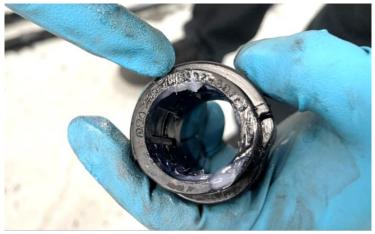
**Step 11** Separate the bushings along the split and wrap them around the sway bar.
