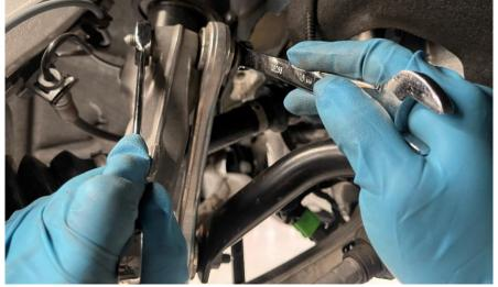
**Step 7** Using a 16mm 12-pt wrench and 16mm wrench, loosen the lower end link hardware.
