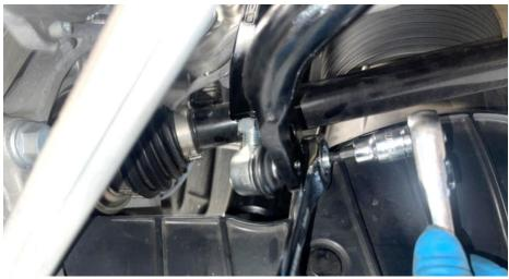
**Step 15** Using a T30, T20 Torx, and 13mm socket, reinstall the front underbody panels.
