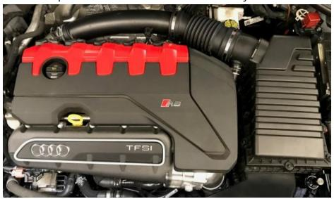
**Step 2**Remove the engine cover.
