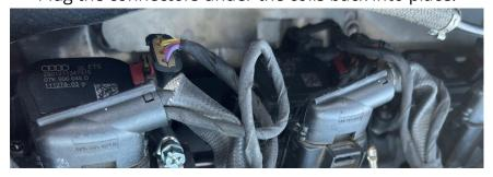
**Step 34**Reconnect the plug below the oil fill neck.
