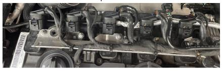
**Step 33**Plug the connectors under the coils back into place.
