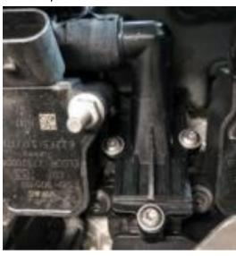
**Step 31**Connect the coil plugs to the coils.
