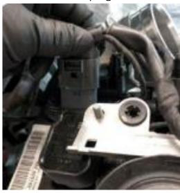
**Step 16**Using a T20 Torx, remove the 3 bolts from the PCV valve.
