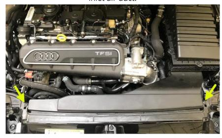
**Step 9**Move duct back, and then up, to remove.
