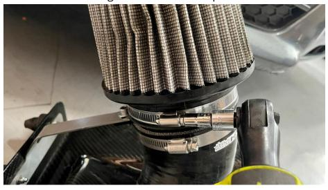
**Step 18**Plug the MAF sensor back into the MAF housing.
