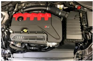
**Step 2**Remove the engine cover.
