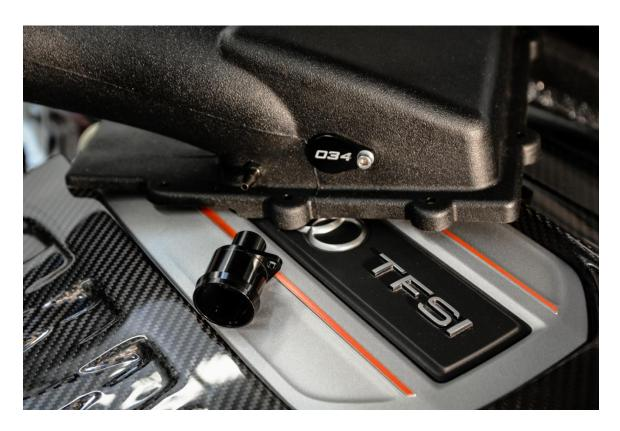
**Step 9** – For Golf, GTI, and A3 owners, mount the SAI provision on the side of the airbox using the provided fitting and allen bolt. Torque bolt to 4 Nm using a 4mm Allen key.
