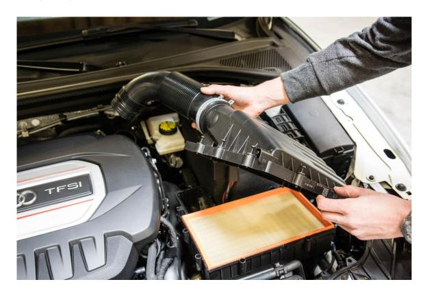
**Step 6** – With the upper air box removed, lift the factory panel air filter from the lower air box.
